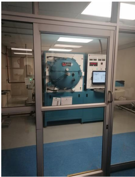
Image: The High Vacuum Heat Treatment Furnace for Titanium Alloys
